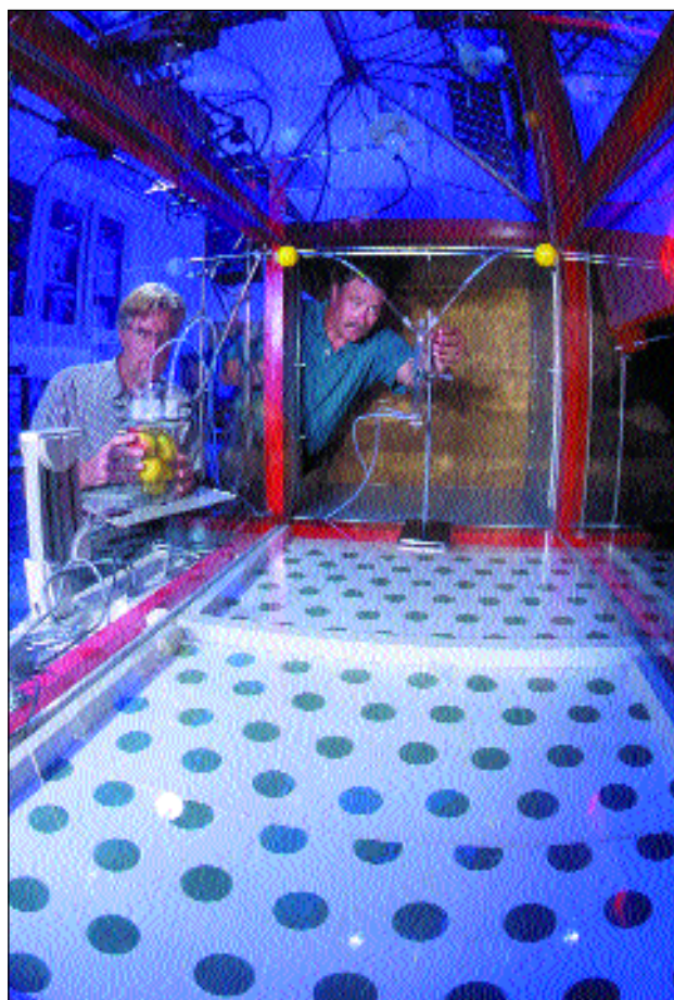
In the laboratory, entomologists prepare a flight tunnel experiment. Insects fly upwind when stimulated by the scent of a pheromone and use the moving spots on the floor as visual cues. (Photo courtesy of Scott Bauer/Agriculture Research Service Photo Unit)
