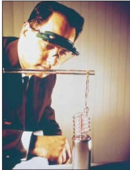
Theodore Maiman with his ruby laser in 1960. The first lasers tended to be bulky and fragile and were prone to overheat. Subsequent work in semiconductors resulted in vastly improved designs. (Hughes Research Laboratories, Inc.)
