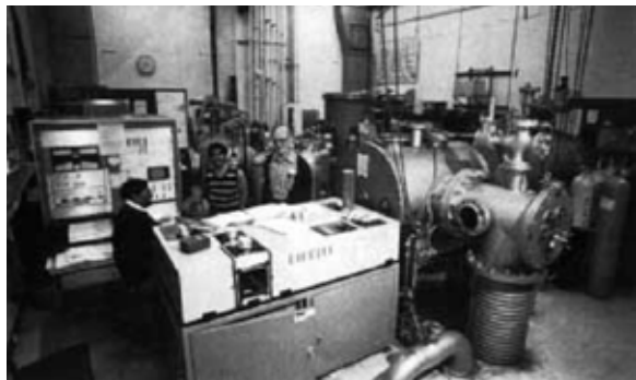
Fenn's "big leak" molecular-beam system, with two 32 inch diffusion pumps and one 16 inch "Jet Booster Pump," after it was moved from Princeton to Yale. Fenn, standing on the right, is accompanied by two postdoctoral fellows, S. B. Ryali, also standing, and S. P. Venkateshan, sitting.
