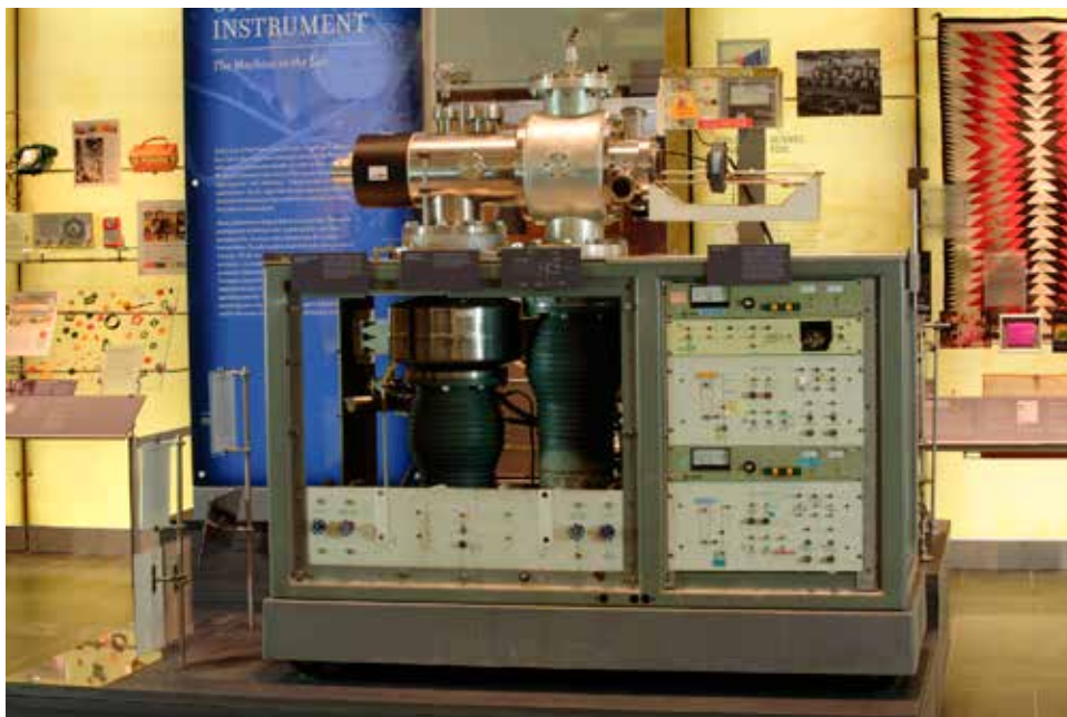
Photograph of Fenn's electro-spray ionization spectrometer apparatus, on display at the Chemical Heritage Foundation in Philadelphia.
