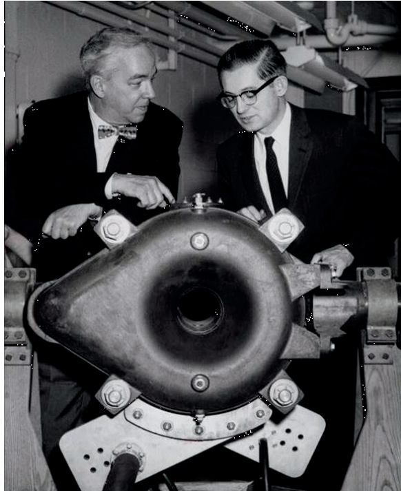
Ben is seen here with Prof. Francis Bitter, reviewing features of Bitter's design for water-cooled solenoid electromagnet. This photograph was (probably) taken in Prof. Bitter's magnet laboratory in the basement of Building 4 on the MIT campus, circa 1957. (The MIT Museum Collections.)
