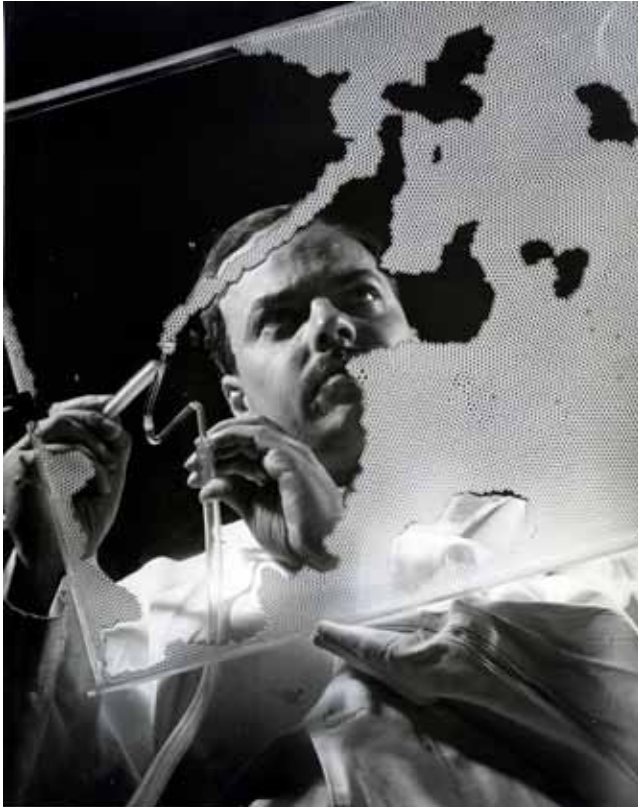
Mullins studies a bubble raft model of a two-dimensional crystal, circa 1956. Evident are grains, grain boundaries, vacancies and surface structure. Photo courtesy William Mullins Jr.
