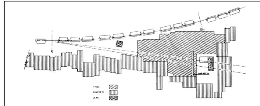
FIGURE 2 The design of the neutrino experiment at the Brookhaven Alternating Gradient Synchrotron.
