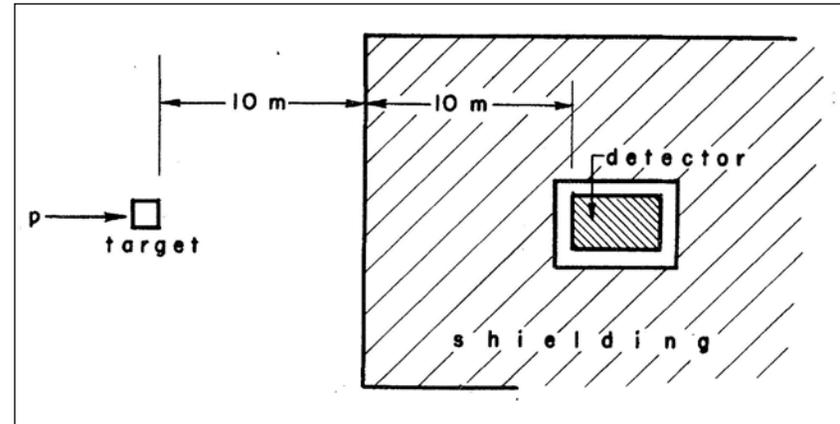
FIGURE 1 Schwartz's initial neutrino beam concept.
