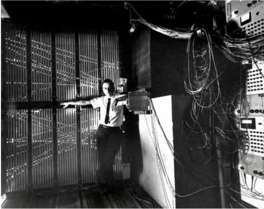
A pleased Mel Schwartz, standing by the spark chambers that he built. The tracks in the spark chambers are a multiple exposure of cosmic-ray muons, which show the same “clean” straight character as muons arising from neutrino interactions.
