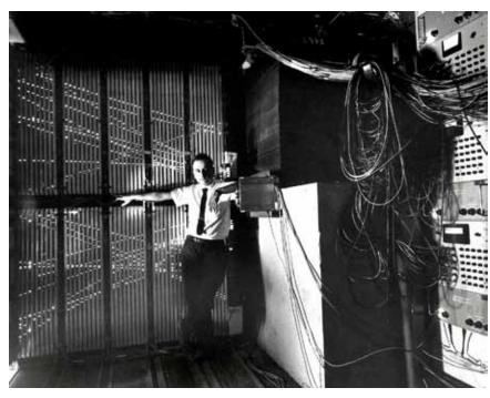
A pleased Mel Schwartz, standing by the spark chambers that he built. The tracks in the spark chambers are a multiple exposure of cosmic-ray muons, which show the same "clean" straight character as muons arising from neutrino interactions.
