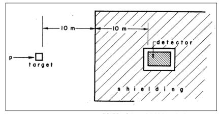
FIGURE 1 Schwartz's initial neutrino beam concept. ≣
