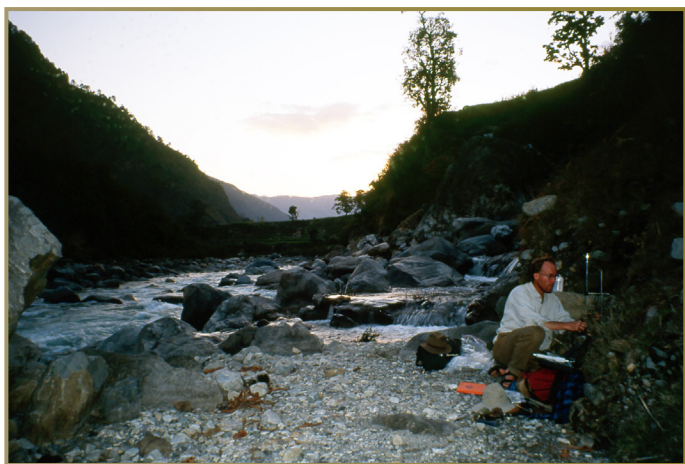
Figure 6 Titrating alkalinity in the field, Nepal. The titrations, water, and sediment samples were used to quantify the contribution of Himalayan rock weathering to marine strontium in the Cenozoic. Photo by Nathan English.
